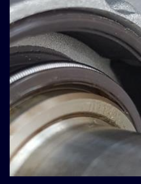
IP67: Radial shaft seal with annular spring on twist-free ground sleeve
